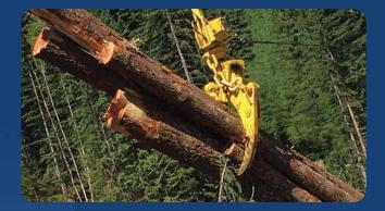
T-MAR Yarding Grapples incorporate a new, innovative design for holding bundles, grabbing tops and minimal line pinching and abrasion.
